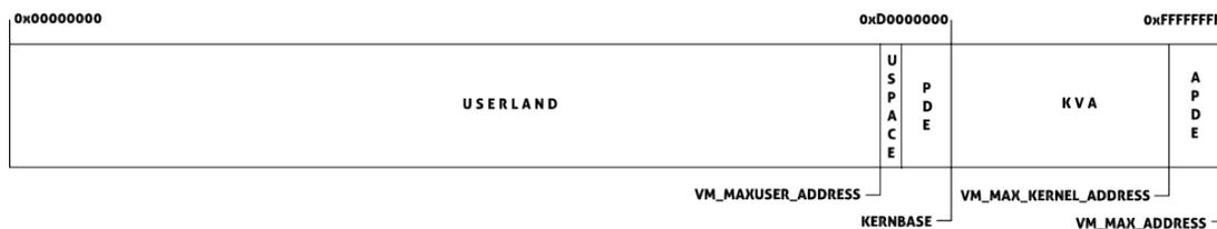
Figure 3.1: Memory layout of OpenBSD on the i386 architecture.
